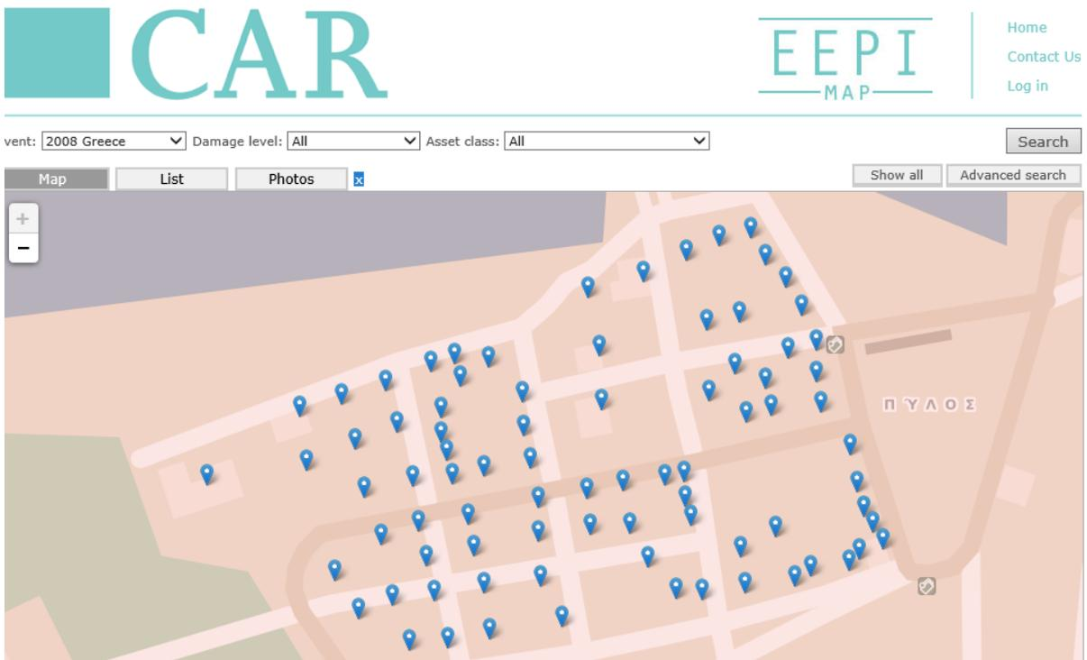
Figure 8: Pylos Vulnerability Street Survey Map (Top); ‘EEPI Map’ photograph location map (bottom). Pylos Survey, June 2008. During the field survey, buildings were assigned a number which was identified on a map (top). This allowed the remote analyst to accurately locate the buildings on EEPI map (bottom) and assign the photographs to the correct location.
